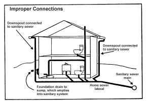
In this example, rainwater is channeled into the sanitary system, greatly overloading the system during periods of rain
