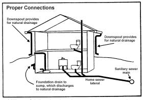
Millions of dollars in otherwise unnecessary upgrades to the sanitary system can be avoided when rainwater is diverted away from the system, as shown above.
